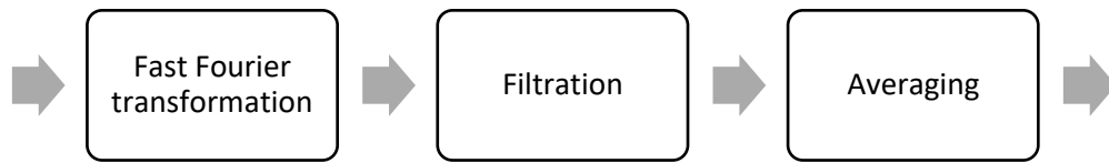
Figure 5. Main stages of vibration signal analysis.
